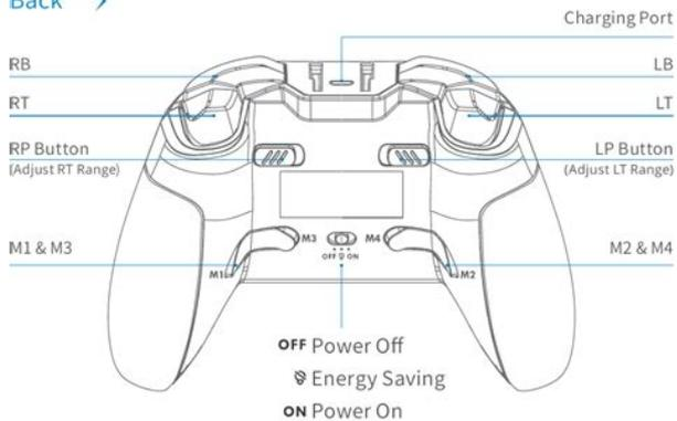
Note: Under Wireless Android Mode, M1 button works also as left button of Air Mouse, Pair button works also as Power Switch of Air Mouse.
